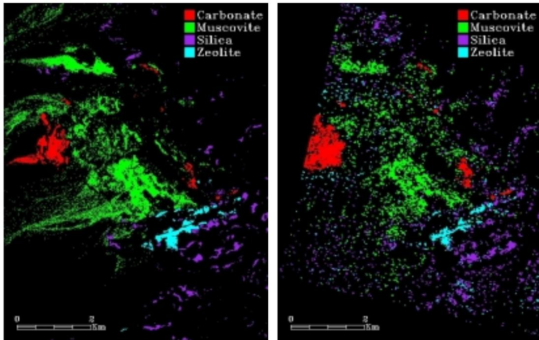
Figure 6: MTMF mineral maps for AVIRIS (left) and Hyperion (right) produced for a subset (combined) of the endmembers in Figure 4 for the northern Death Valley, California and Nevada site. Colored pixels show the spectrally predominant mineral group at concentrations greater than 10%.
