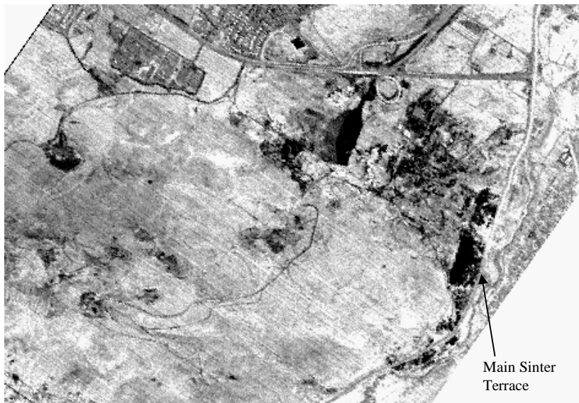
Figure 2: Steamboat, Nevada, 1996 TMS results. Dark areas represent high silica concentrations
