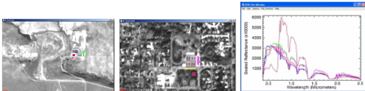
Figure 1: Left is geocorrected AVIRIS grayscale image (Band 31, 0.66 micrometers) of the Boulder Rifle Club site with colored ROIs overlain. ROIs were selected based on field measurements. Red is a gravel/sand parking lot (Gravel #1). Green is a sandy gun-range gravel (Gravel #2). Blue is a galvanized metal building. Center is geocorrected AVIRIS grayscale image (Band 31, 0.66 micrometers) of the Centennial Middle School site with colored ROIs selected based on field measurement sites overlain. Magenta is a sandy gravel parking lot. Sea Green is a yellow school bus. Yellow is an asphalt driveway. Maroon is a green grassy athletic field. Purple is the green portion of a synthetic tennis court surface. Orange is the red portion of a synthetic tennis court surface. Right is spectral plot of selected Mean AVIRIS Radiance Spectra (Rifle Club gravel #1, gravel #2, galvanized building and Centennial Middle School sandy gravel parking lot and green grassy athletic field) with colors matching ROI overlay colors.
